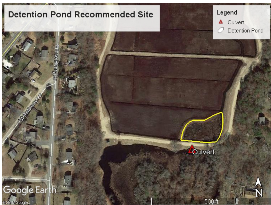
Figure IV-1 Recommended location for a detention pond above the Mill Pond culvert to prevent particle and macrophyte debris transport. Site is part of the existing bog system.
