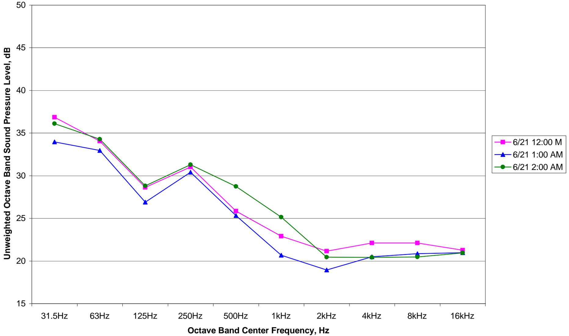
Figure 6. LT-1 One-hour Octave Band L90, Nighttime, Turbine Off, Hub Wind 3.6 to 4.8 m/s
