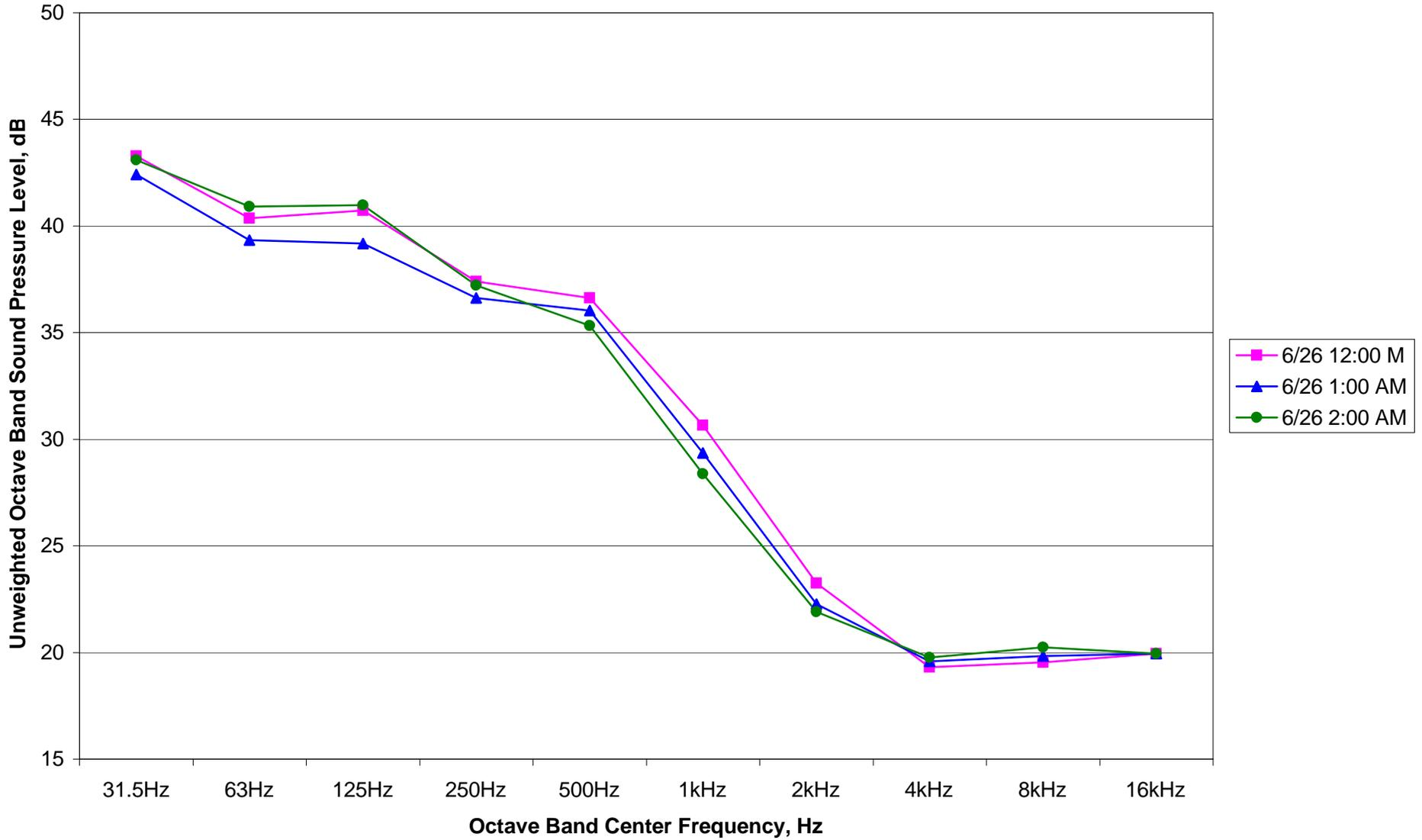
Figure 5. LT-1 One-hour Octave Band L90, Nighttime, Turbine Running, Hub Wind 3.2 to 3.8 m/s
