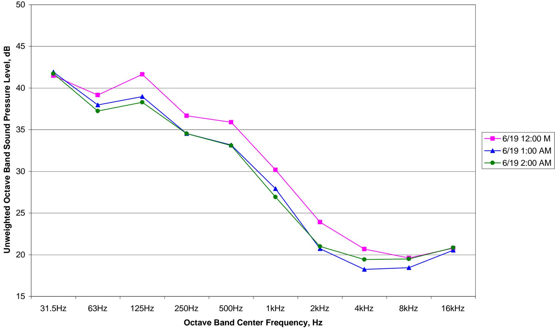
Figure 4. LT-1 One-hour Octave Band L90, Nighttime, Turbine Running, Hub Wind 7.0 to 7.6 m/s
