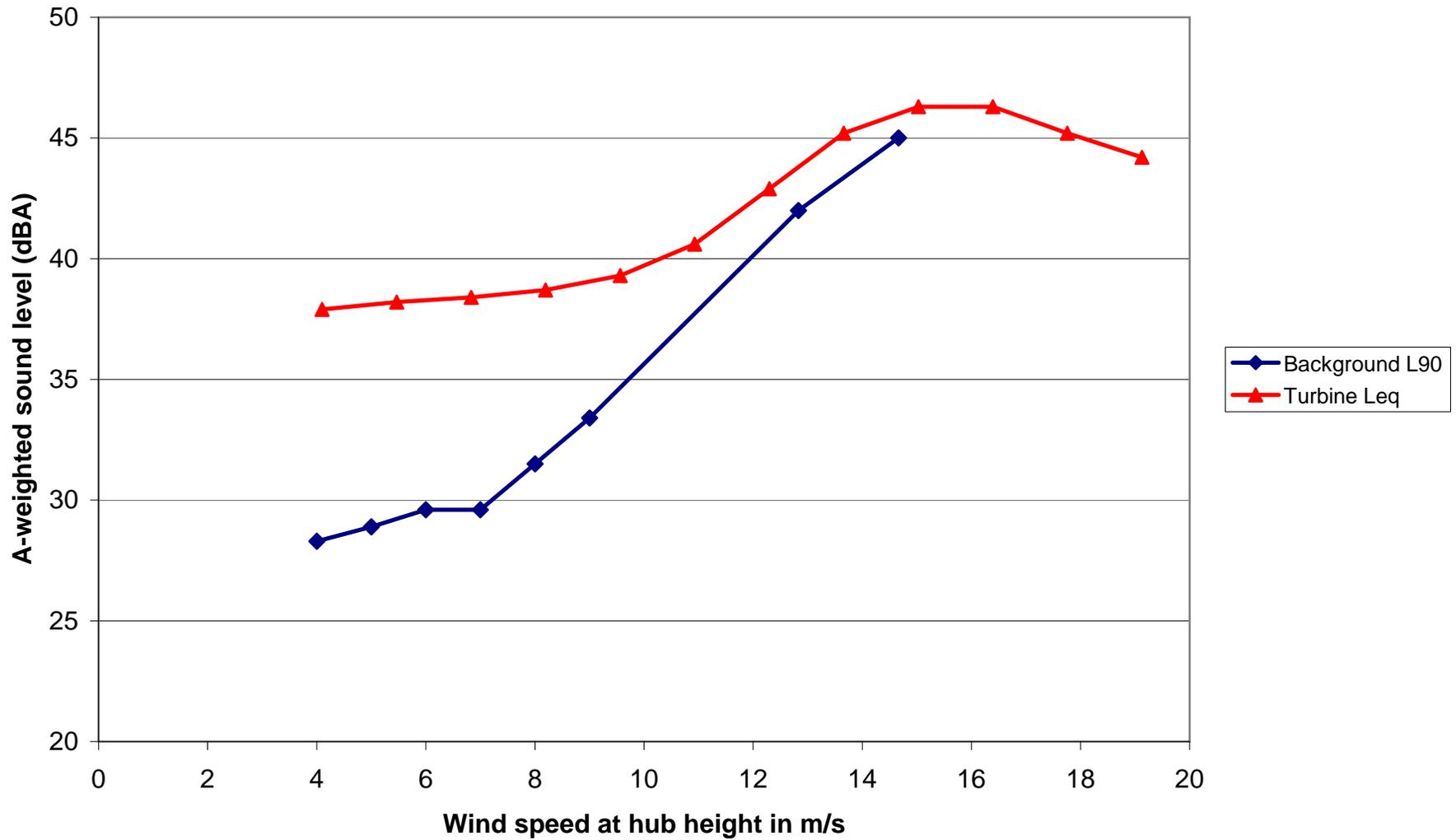
**Table 7. Falmouth Wind1 & Wind2 noise levels compared with ambient background sound levels at different wind speeds**
