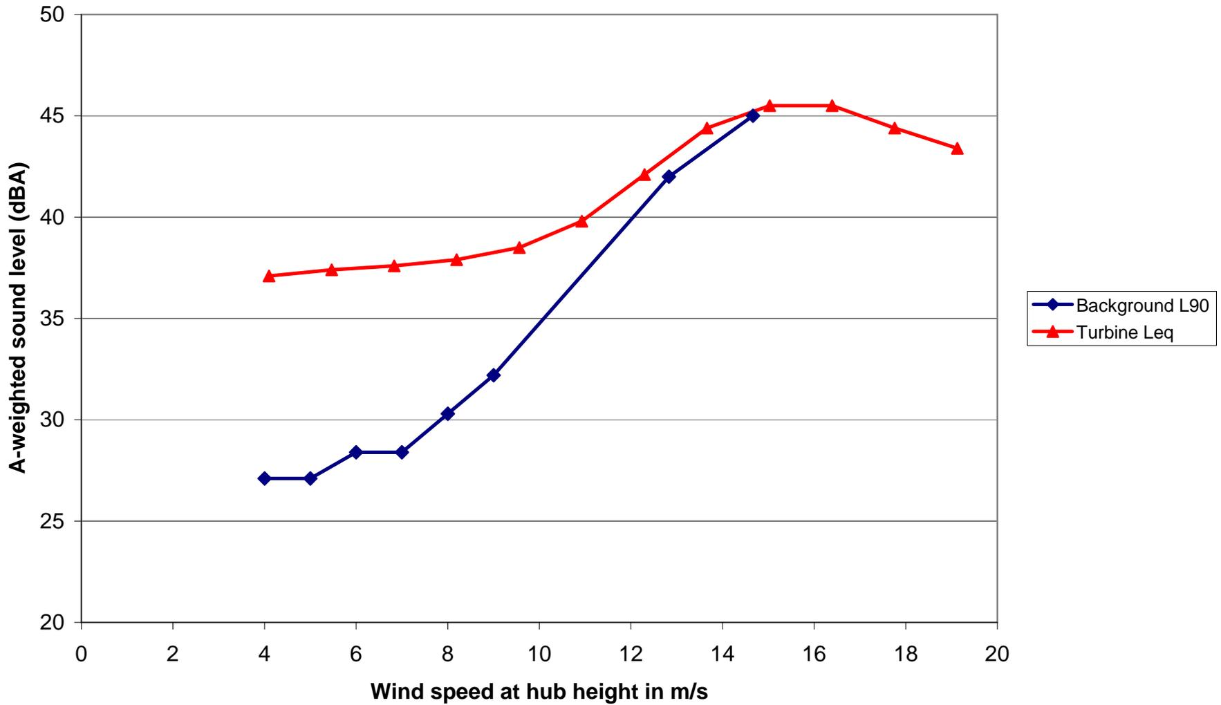
**Figure 8. LT-2: Lowest Background L90 and Computed Wind-1 + Wind-2 Turbine Leq Sound Levels as a Function of Hub Wind Speed**
