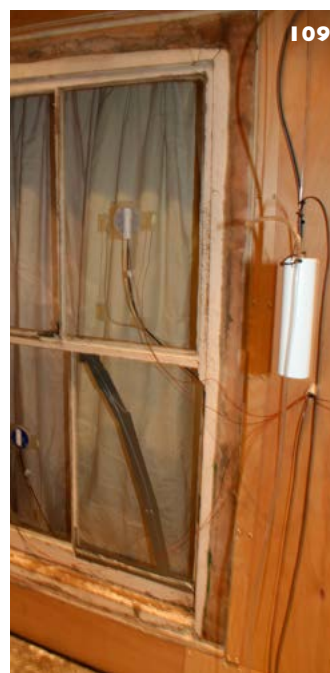
108 & 109: Testing windows in the climate chamber at Glasgow Caledonian University.
