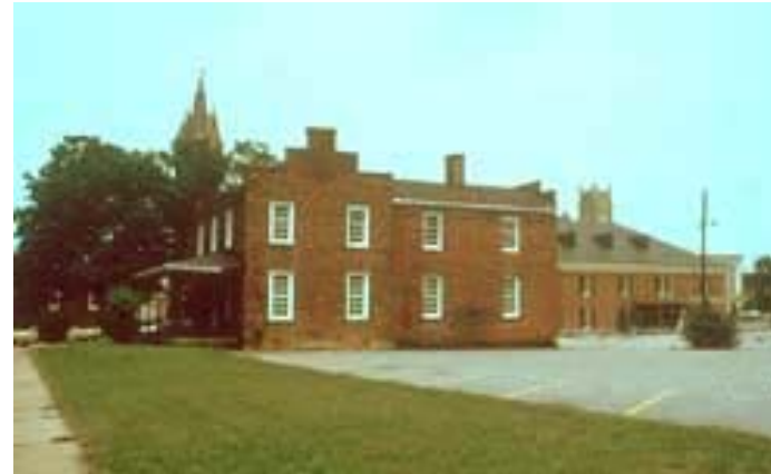
E.g. where site work is incompatible – new parking extends to edge of building and changes setting.
