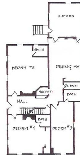
First floor plan, after rehabilitation. Alterations to intact spaces at the front of the first floor (hall, parlor, dining room) destroyed the spatial symmetry characteristic of the formal 18th-century interior design.
